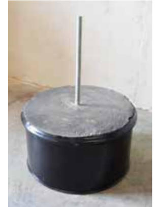
Foot mounting made with steel drums and concrete
