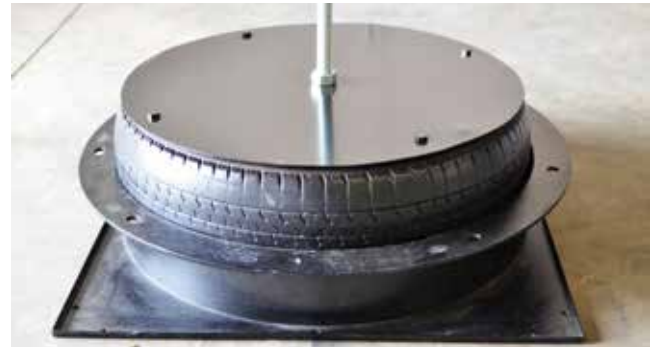
Green Anti-vibration Mountings for fans using discarded car tyres
